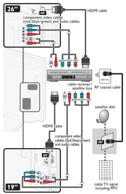
You can also connect this unit to the cable receiver or satellite box other than the HDMI or the Component Video output jacks or Composite Video output jack (**\*\*\* p.37, 38**) because they might have different output jacks.
