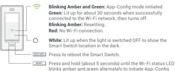
Press and hold (about 10 seconds) until the Wi-Fi status LED blinks amber rapidly to factory reset the Smart Switch.
